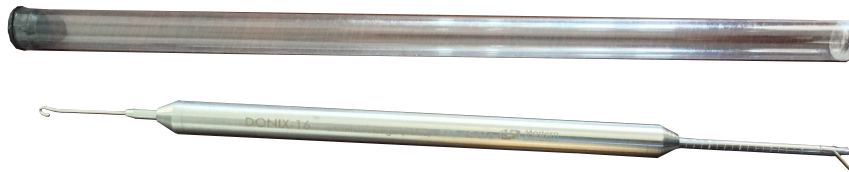
Dontrix Gauge for Tension and compression force measurement of upto 16 Oz Cat.No..... AC-254
